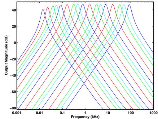
**Fig. 9.** Frequency decomposition (sub-band processing) can be achieved on the test-bed FPAA by using the  $C^4$  bandpass filter block in each CAB. Here the center frequency of the  $C^4$  is shown to be programmable over a wide range of frequencies.
