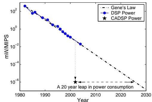
**Fig. 1.** Data from [1] showing the power consumption trends in DSP microprocessors along with data taken from a recent analog, floating-gate integrated chip developed by the CADSP team.
