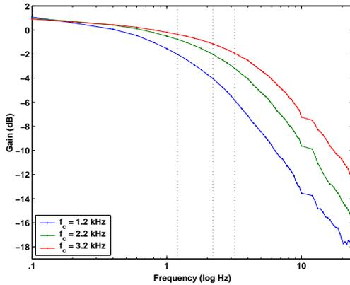
**Fig. 6.** Here, the frequency response of the source–follower circuit is shown for several bias currents. An internal floating–gate transistor is used as a current source to set the OTA’s bias. Injecting the floating–gate device, increases the current and thus the bandwidth of this first order filter.
