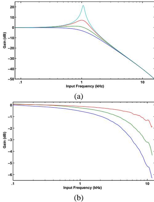
**Fig. 8.** The simulated (a) and experimental (b) frequency response of a second-order section filter is shown here. The Q parameter is adjusted by increasing the bias current of the positive feedback amplifier via a floating-gate current source.
