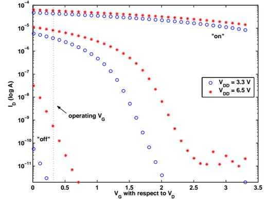
**Fig. 3.** Floating-gate switches can be programmed within a wide range. Here, examples of an “on”, “off”, and mid-position device are shown. During programming, currents are measured with  $V_{DD} = 3.3V$  for large currents and  $V_{DD} = 6.5V$  for small currents. This effectively extends the programming range of the device.
