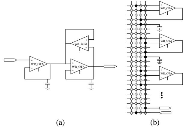
**Fig. 7.** (a) A second–order section filter can be implemented with two OTAs in a source–follower configuration and a third OTA that creates positive feedback. (b) Using the switch matrix, two OTAs within the CABs are connected in a second–order section configuration. The programmable biases shown in Figure 5(a) are not included here for simplicity, but each OTA has a current mirror and floating–gate current source that sets its bias.
