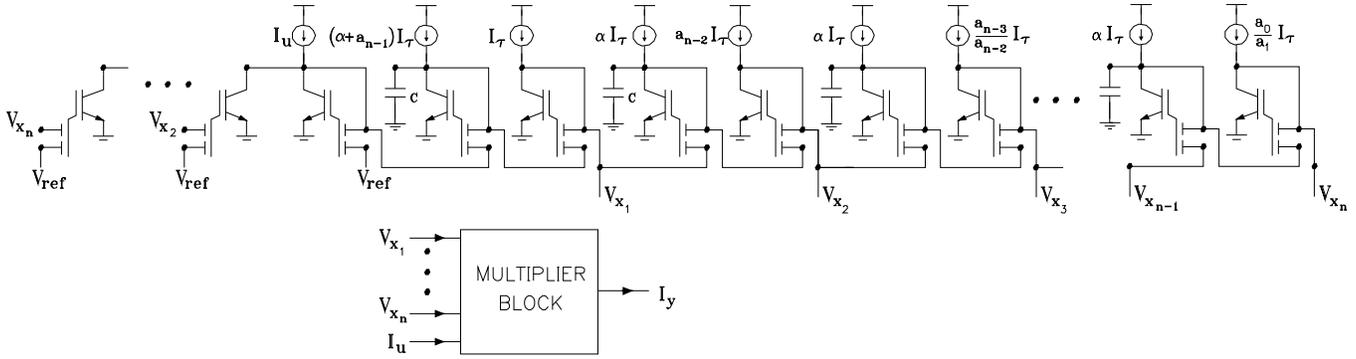
Fig. 2. A generic shifted-companion-form filter. It can be used to generate any linear transfer function. The poles and zeros can be tuned using the bias currents. The multiplier block is implemented as described in Section IV.
