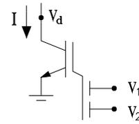
Fig. 3. Symbol for a 2-input Multiple Input Translinear Element (MITE). Ideally, it should obey the law  $I = I_s \exp(\frac{\kappa}{U_T}(V_1 + V_2))$ .
